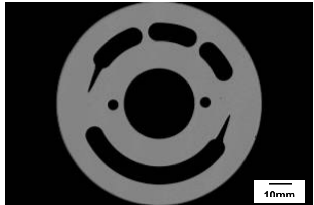
Fig. 3 Scanning ultrasonic reflectoscope image of port plate after load test.
