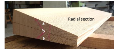
Image of sawing into top plate (left). Timber cut for cello top plate (right)
