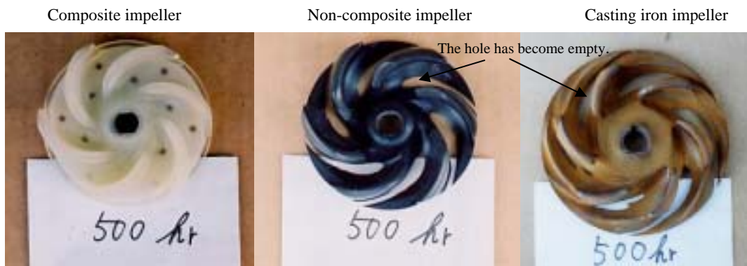
Fig.6 Abrasion photograph of impeller at pump running in slurry tank
