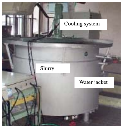
Fig. 2 Photograph of the slurry tank for the pump durability examination
