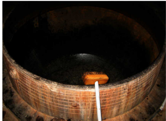
Fig.3-4 After dilute hydrochloric acid treatment.
