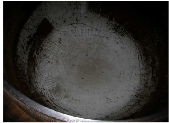
Fig.3-2 After citric acid treatment.
